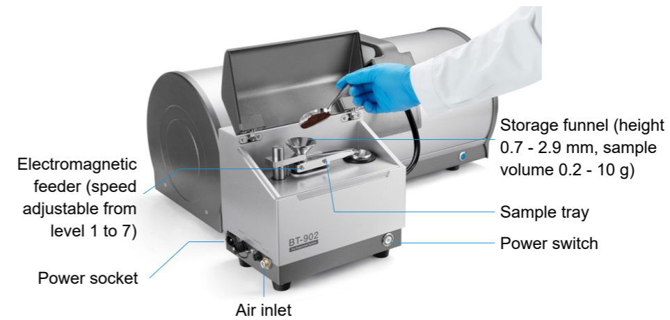
BT-902 Automatic Dry Dispersion Module
