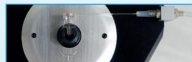
Connections to the cantilever. A connector matching the reservoir end of all CytoClips models connects to the pressure controller via standard tubing.
